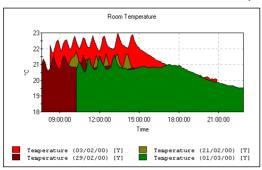
In this type of chart, the values of points are plotted against the time at which they were recorded, and the area under the plot is shaded.
