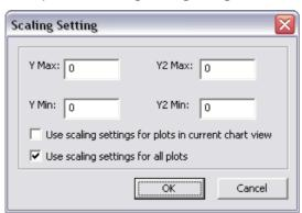
This allows you to manually set any arbitrary value for the Maximum and Minimum Y-axis values.
