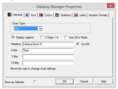
The properties controlled by this dialog are grouped into 6 sections. The 'tabs' at the top on the **Properties** dialog are used to move between those groups.
