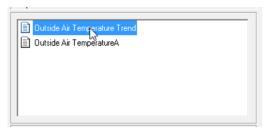
Select a chart to open in the file list box. This lists all the files of the type selected in the Types box, that are associated with the targeted controller.
