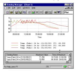
The Statistics Window can be adjusted by dragging the separator bar up or down to display statistics for more or fewer datalog plots at one time. The display can be adjusted so fewer statistics are displayed, see *Selecting the types of statistics for display* on page 52.
