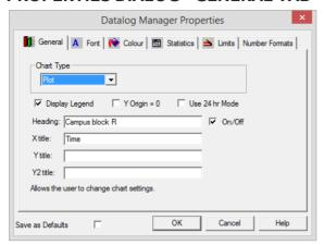
This tab in the Datalog Manager Properties dialog sets the format for the current chart, and allows you to change display options of the current chart.
